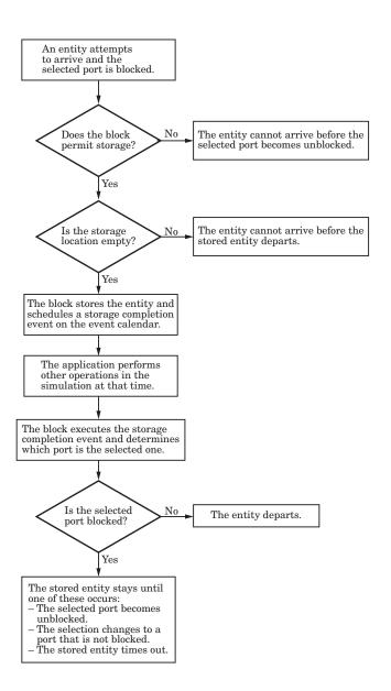
**Note:** This block permits storage only if you set **Switching criterion** to From signal port p, and then select **Store entity before switching**.
