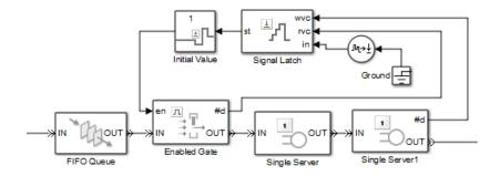
**Note:** The IC block in the Simulink library set operates in a time-based manner and is not suitable for event-based signals.
