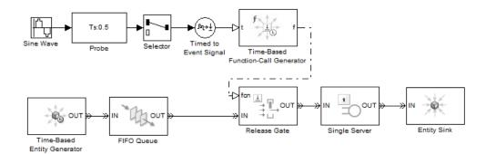
In this model, the **Event generation mode** parameter of the Time-Based Function-Call Generator block is set to Period from port. The Probe block detects the sample time of a sine wave signal and connects it to the input port t of the Time-Based Function-Call Generator block. The value at the input port t determines the period — or time delay — between successive function-call events generated by the block and is used to control entity advancement through the Release Gate block.
